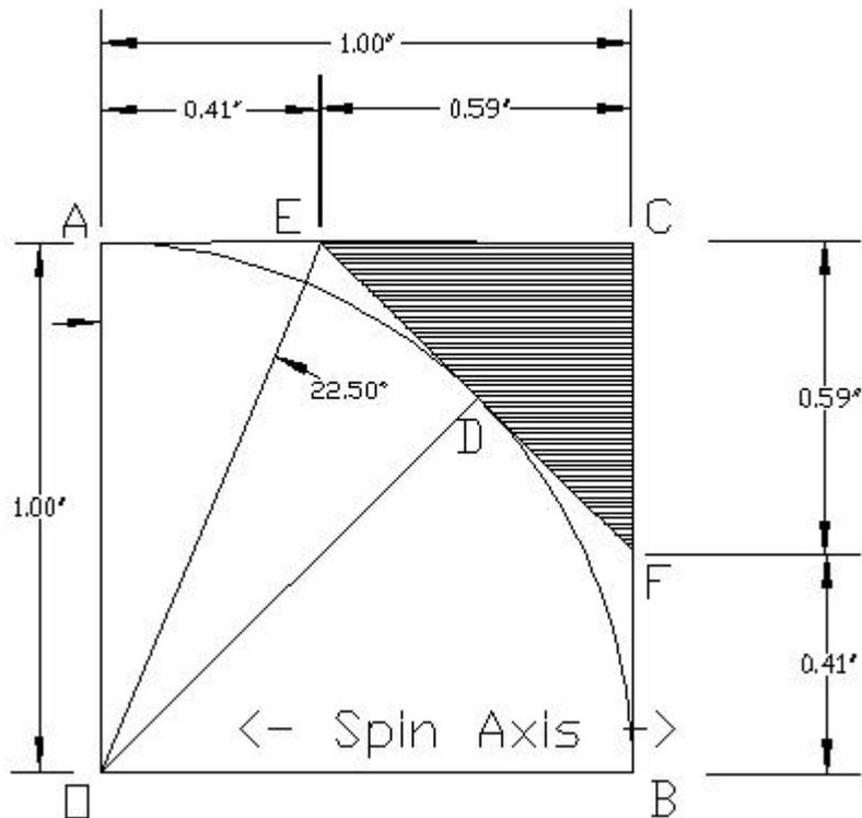
Figure 1 shows the layout for the first cut. The length of AE is  $\tan(22.5)$  or 0.41". Because of symmetry, BF also is 0.41"
